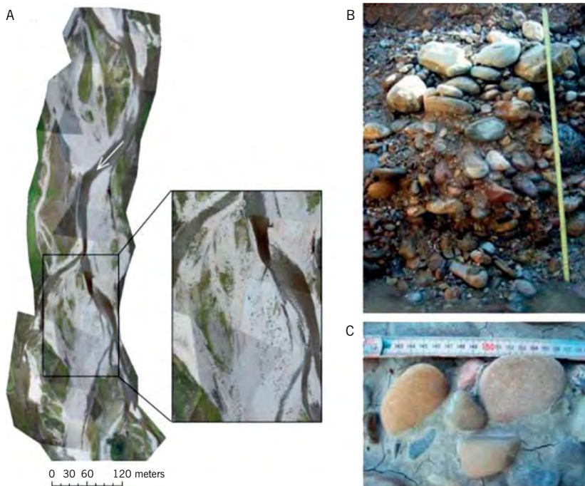
Figure 3.1: A) A mountain reach with a complex architecture including riffles, pools, central bars and secondary channels (Feshie River, Scotland, UK; arrow shows flow direction). The inset zoom shows how morphological complexity changes in relation to the scale in which it is investigated. B) Sediments are mixed horizontally and vertically: Gravel and cobble sediments in a complex arrangement (Ribera Salada, Southern Pyrenees). C) Fine sediments deposited during low flows clog the spaces between gravel particles (Isábena River, Southern Pyrenees)
