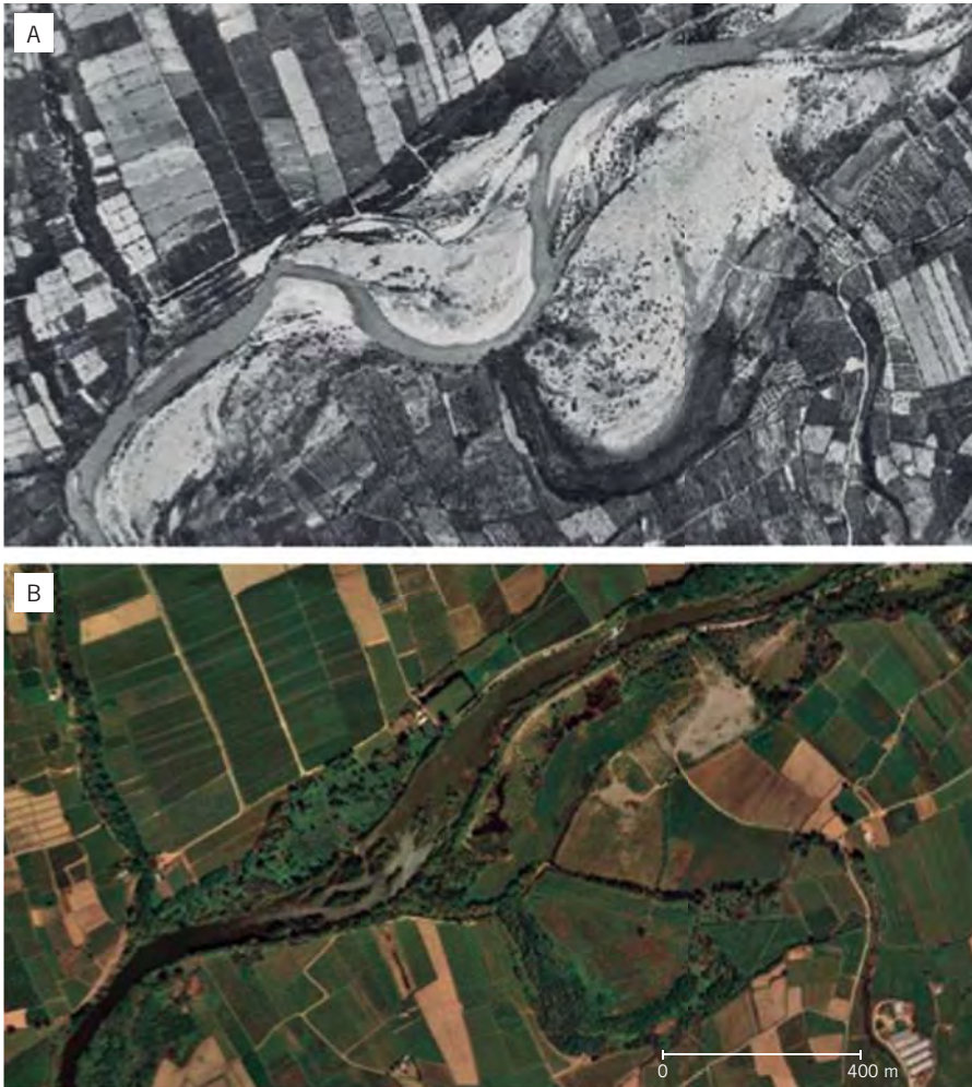
Figure 3.7: Channel narrowing and vegetation encroachment as a consequence of dams in Segre River near the Alcarràs (Ebro basin, NE Spain). A) Segre River, 1956; B) Segre River, 2009
