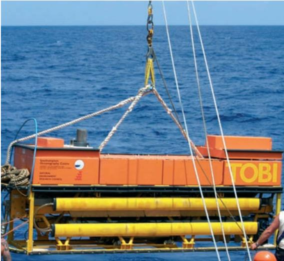
**Photo 3.10: TOBI (Towed Ocean Bottom Instrument) is one of the UK deep sidescan sonars used to produce acoustic maps of the deep seafloor**
