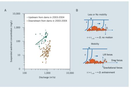
*Note:* v =flow velocity,  $D_i =$ particle of an *i* diameter,  $\tau =$  shear stress,  $t_{c-D_i} =$  critical shear stress for a given particle size *i*.
